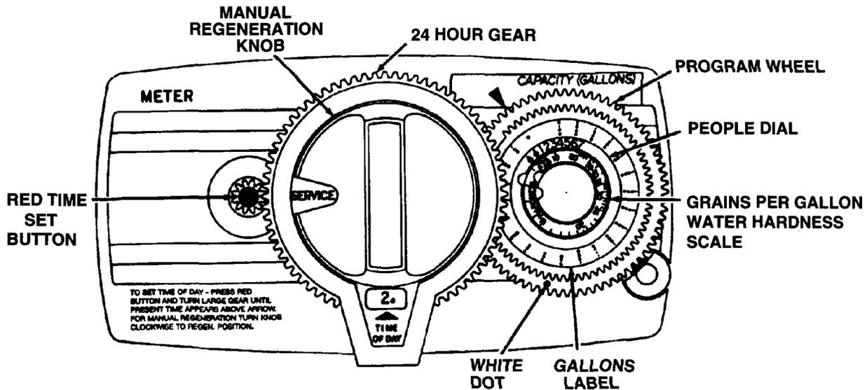
1. Manually index the softener control into the service position and let water flow into the resin tank. When the water flow stops, open a softened water tap until all air is released from the lines, then close the tap.
