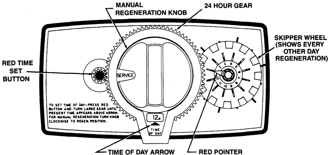
1. Manually index the softener control into the service position and let water flow into the resin tank. When the water flow stops, open a softened water tap until all air is released from the lines, then close the tap.
