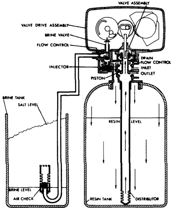
Hard water enters the unit at the valve inlet - flows around the lower piston groove - down thru the top of tank passage - downward thru the resin - up the distributor tube - thru the center hole in the piston - over the top edge of the piston and out the drain line.
