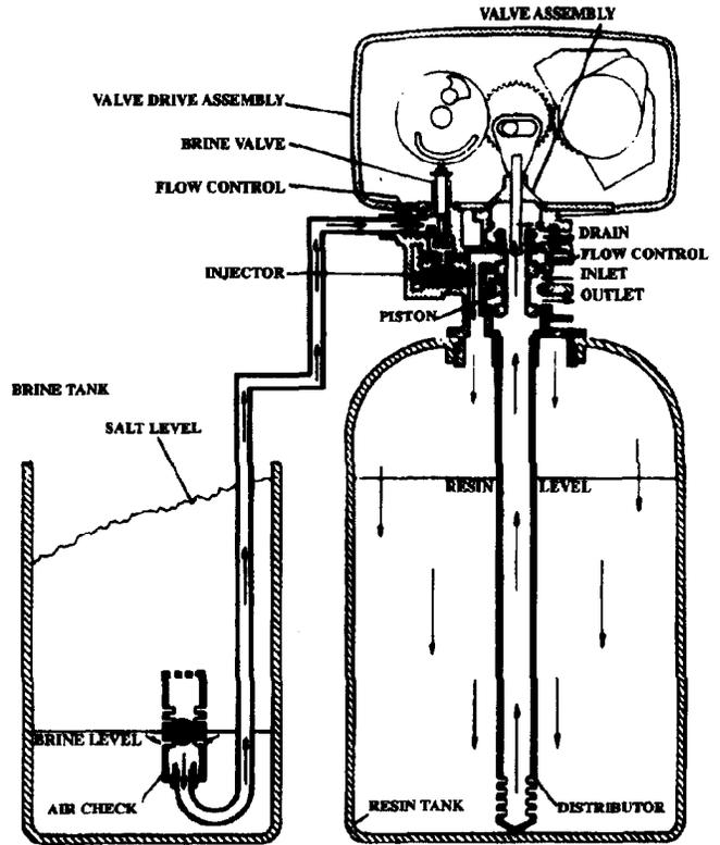
Hard water enters the unit at the valve inlet - flows around the lower piston groove - thru the injector nozzle and orifice to draw brine from the brine tank. The brine flows down thru the resin - into the distributor - up thru the center tube - thru the center hole in the piston and out the drain line.
