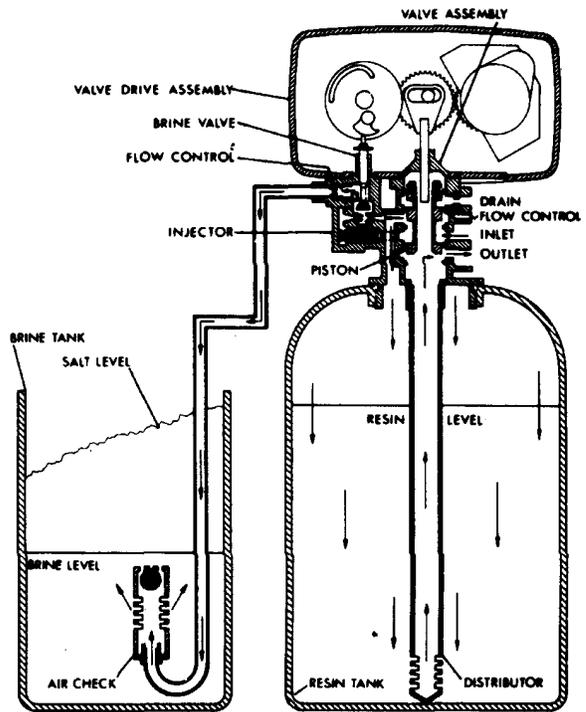
Hard water enters the unit at the valve inlet - flows around the lower piston groove - thru the injector throat - thru the brine valve and flow control to fill the brine tank. Hard water also flows around the lower piston groove - thru the passage to the top of tank - down thru the resin and enters the distributor as conditioned water. The conditioned water flows up thru the center tube to the valve outlet.
